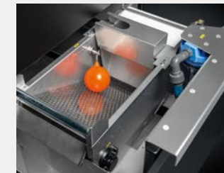
Automatic waste separation in the chip conveyor
